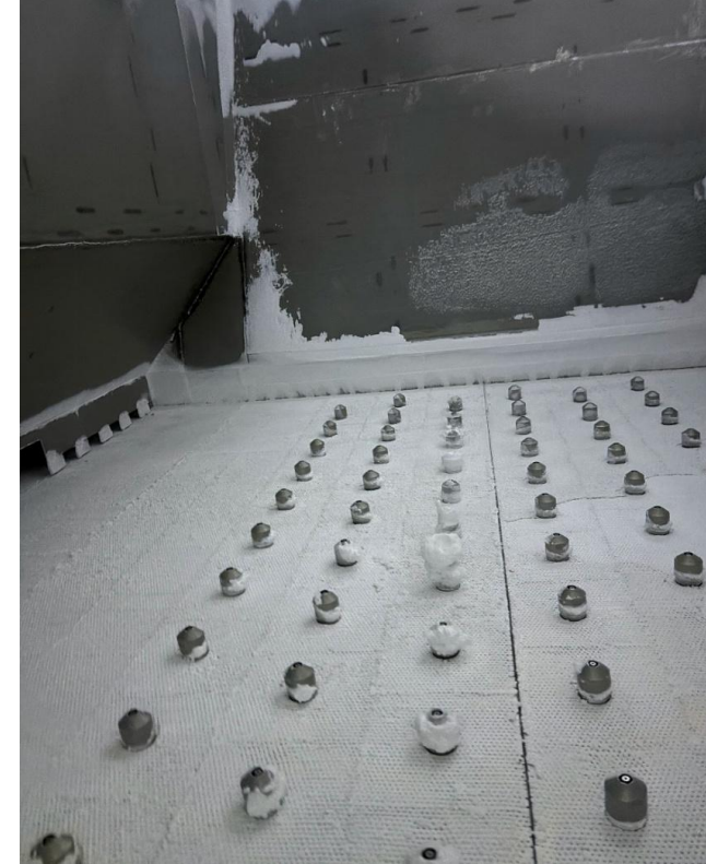
Fouling in the granulator fluidization plate in all compartments
